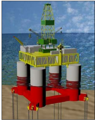
Tension Leg Platform
