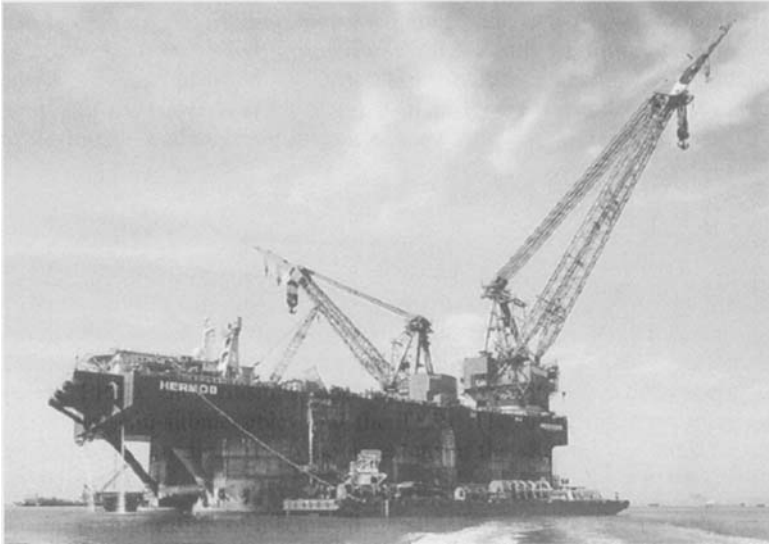
Figure 7.136 Semi-submersible crane vessel (Heerema Offshore)
