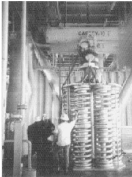
Figure 7.12 Passive spring riser tensioner for Prince TLP (from Koon, et al 2002)
