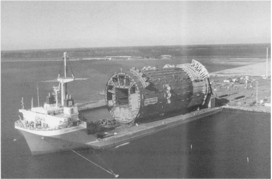
Figure 7.135 Offloading of spar hull for transport (Dockwise Shipping B.V., www.dockwise.com )
