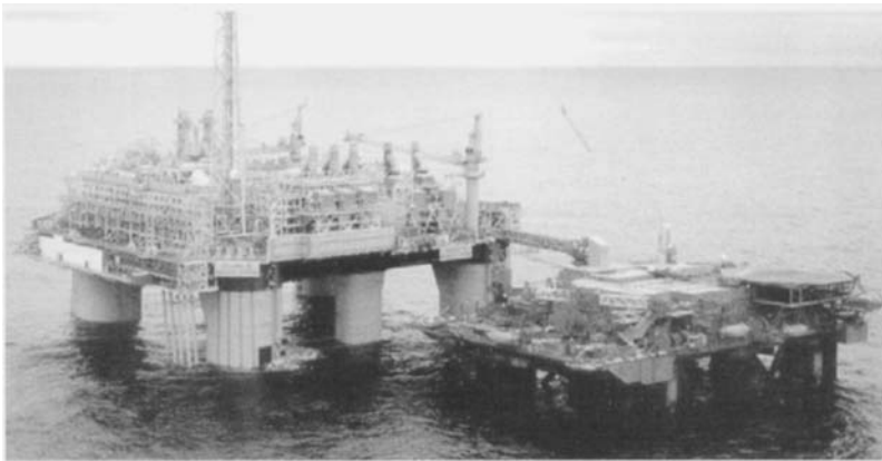
Figure 7.9 Asgaard “B” semi-submersible with single level integrated deck (Øyvind Hagen, STATOIL)
