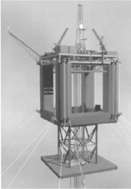
Figure 2.8 Deep Draft Submersible (DDS) (Reproduced courtesy of Technip)
