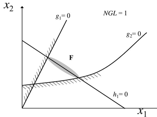
$$\begin{aligned} &\min f(x_1, x_2) \\ &\text{s.a.: } h = 0 \\ &\quad g_1 \leq 0 \\ &\quad g_2 \leq 0 \end{aligned}$$
