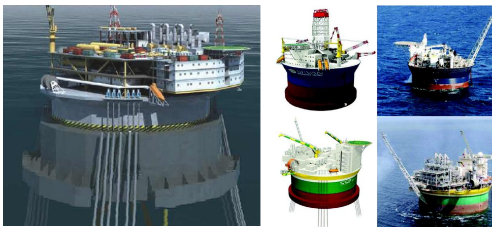
Figure 1 – Monocolumn platforms. Left: MonoBR-GoM, (Nishimoto et al, 2010), with a moon-pool. Right up: FPSO Sevan 1 Hummingbird; bottom: FPSO Sevan Piranema, (Gonçalves et al, 2010b).
