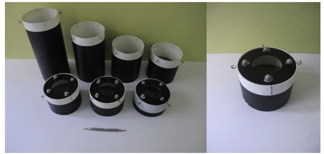
Fig. 3. Illustration of PVC models of the cylinders with low aspect ratio.
