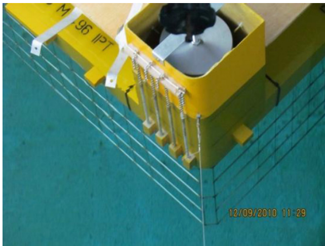
Fig. 8. Picture of the semi-submersible model scaled in 1:100 with external damping simulator.
