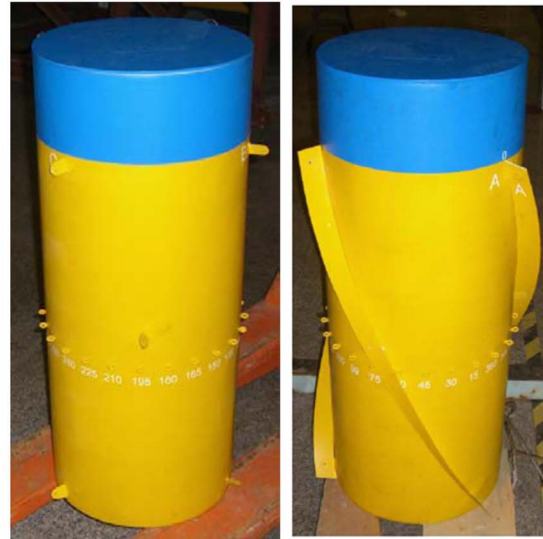
Fig. 10 Comparison between results for spar model bare hull and hull with strakes by Wang et al. [16]
