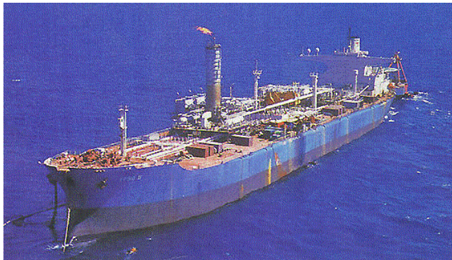
Figure 1: A FPSO at Marlim 2 Basin (Petrobras/Brazil). Single Point Mooring at stern.
