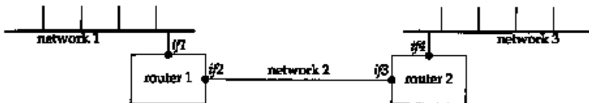
Figure 8.3 Identification of interfaces printed by traceroute.
