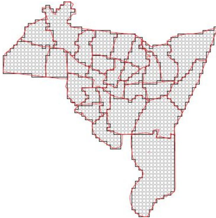
Figure 5.14 Converting from rasters to polygons and points, with the original polygon data in red
