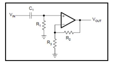
$$A(s) = \frac{1 + \frac{R_2}{R_3}}{1 + \frac{1}{\omega_c R_1 C_1} \cdot \frac{1}{s}}$$
