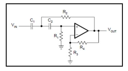
$$A(s) = \frac{\alpha}{1 + \frac{R_2(C_1 + C_2) + R_1C_2(1 - \alpha)}{\omega_c R_1 R_2 C_1 C_2} \cdot \frac{1}{s} + \frac{1}{\omega_c^2 \, R_1 R_2 C_1 C_2} \cdot \frac{1}{s^2}}$$
