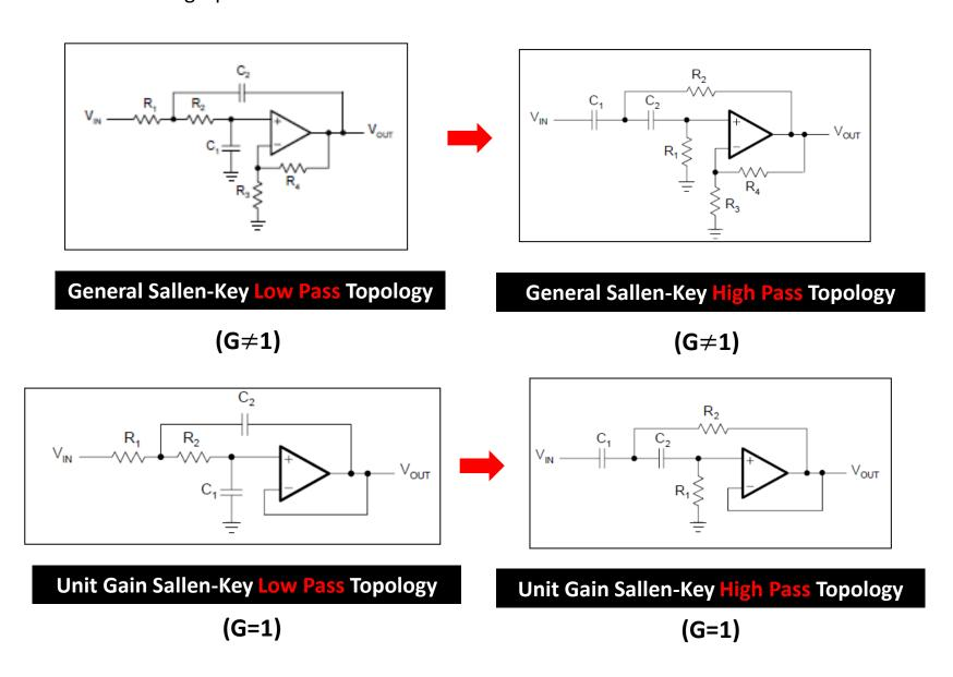
To plot the gain response of a high-pass filter mirror the gain response of a low-pass filter replacing  $\Omega$  with  $1/\Omega$  and s with 1/s
