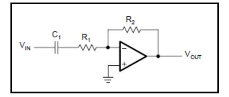
$$A(s) = -\frac{-\frac{R_2}{R_1}}{1 + \frac{1}{\omega_c R_1 C_1} \cdot \frac{1}{s}}$$
