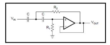
$$A(s) = \frac{1}{1 + \frac{2}{\omega_c R_1 C} \cdot \frac{1}{s} + \frac{1}{\omega_c^2 R_1 R_2 C^2} \cdot \frac{1}{s^2}}$$
