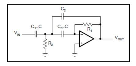
$$A(s) = -\frac{\frac{C}{C_2}}{1 + \frac{2C + C_2}{\omega_c R_1 C C_2} \cdot \frac{1}{s} + \frac{2C + C_2}{\omega_c R_1 C C_2} \cdot \frac{1}{s^2}}$$
