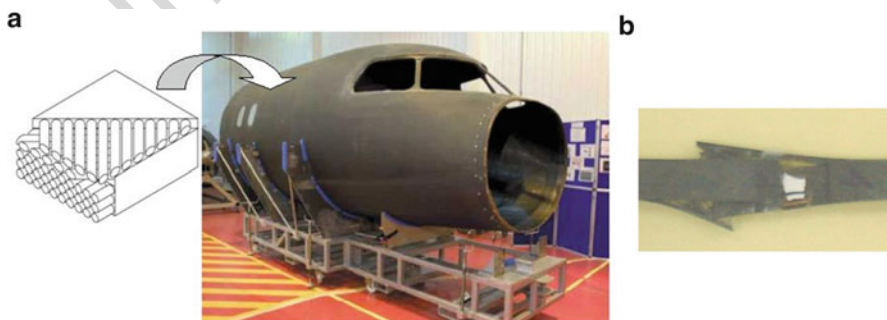
Fig. 1 Composite material: (a) fuselage made of laminate composite; (b) damage and failure in laminate composite materials
