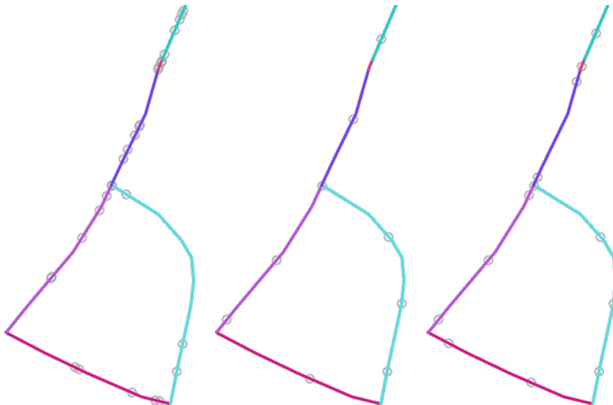
Figura25.43: Five points per line feature, left : min. distances = 0, middle : min.distances != 0, right : min. distance != 0, global min. distance = 0
