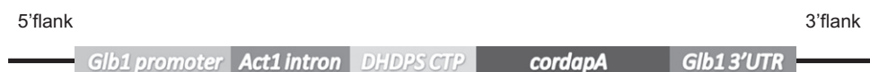
FIGURE 13.8 Organization of the T-DNA cassette for the cordapA gene from Corynebacterium glutamicum , which encodes the bacterial enzyme dihydrodipicolinate synthase. This cassette is integrated into the genome of maize to enhance lysine biosynthesis. Glb1 promoter: Zea mays globulin 1 promoter; Act1 intron: rice actin-1 intron; DHDPS CTP: Zea mays dihydrodipicolinate synthase chloroplast transit peptide directing the gene product to the plastid; cordapA : gene encoding Corynebacterium glutamicum dihydrodipicolinate synthase; Glb1 3'UTR: Zea mays globulin 1 3' untranslated region to terminate transcription.
