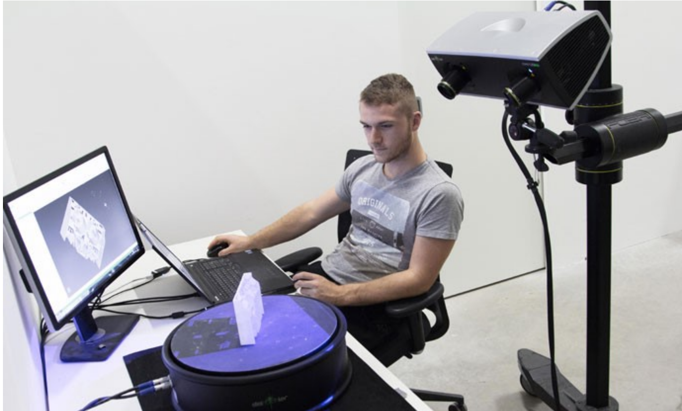
ZEISS COMET L3D 2 - ultra-compact 3D sensor
