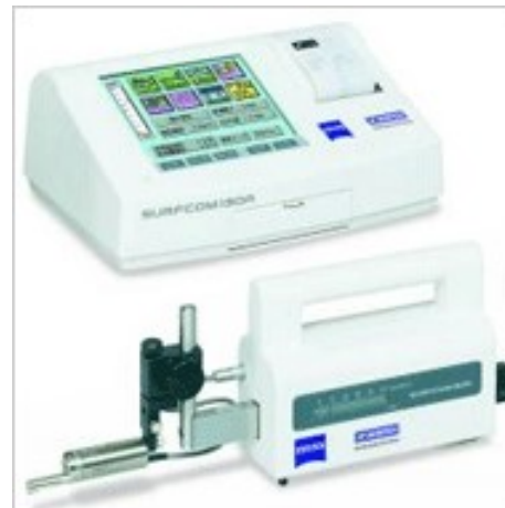
Surfcom 130: Compact Field Surface Texture Measuring Instrument.
