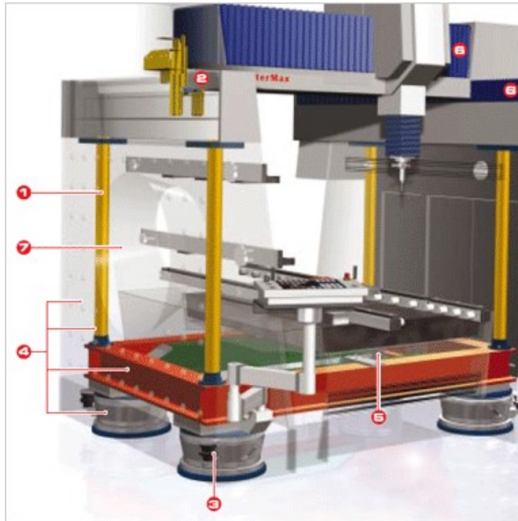
Take a look inside: (1) Invar carriers, (2) Bearing and scale covers, (3) Active anti-vibration system, (4) Dynamic and thermal damping thru TRF, (5) Liquids drainage, (6) Raised guideways, and the (7) Mineral cast.
