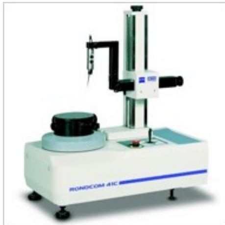
Rondcom 41: Compact desktop model with high-end analysis functions.
