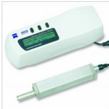
Handysurf E35A: The small, portable surface measuring unit.
