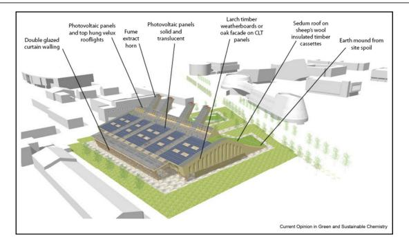
The design and important features of the GSK Carbon Neutral Laboratories. The building is constructed largely of sustainably sourced wood and the use of concrete has been minimized. The orientation and profile of the building is designed to harness the prevailing wind to assist extraction from the fume cupboards. For a virtual tour of the partly complete building see Ref. [17].
