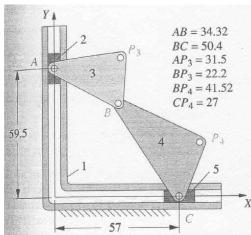
Resp.: a)  $\theta_{AB} = -29,9^\circ$ ,  $\theta_{BC} = 122,8^\circ$ ,  $x_B = 29,7$  mm,  $y_B = 42,4$  mm
