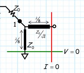
The admittance of a 1/8 short-circuit stub is:
