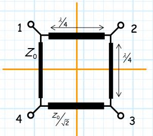
To determine the scattering parameters  $S_{11}$ ,  $S_{21}$ ,  $S_{31}$ ,  $S_{41}$ , of this network, a matched source is placed on port 1, while matched loads terminate the other 3 ports.
