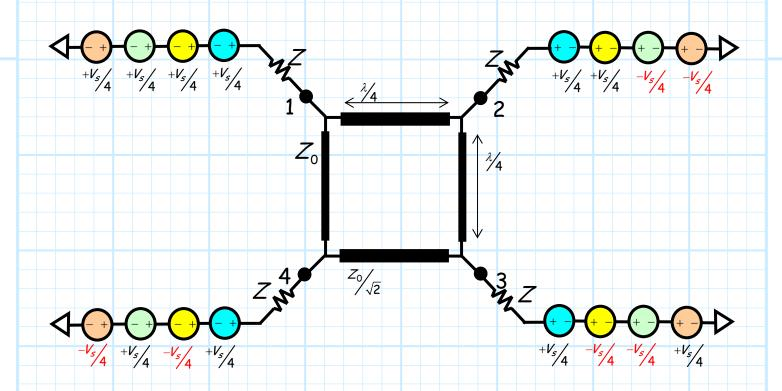
Note that the four series voltage sources on port 1 add to the original value of  $V_s$ , while the series source at the other four ports add to a value of **zero**—thus providing short circuit from the passive load  $Z_0$  to ground.
