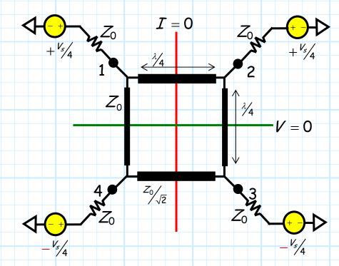
For mode B, the even symmetry exists about the vertical circuit plane, while odd symmetry occurs across the horizontal plane.
