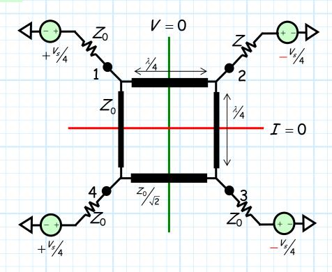
For mode C, odd symmetry exists about the vertical circuit plane, while even symmetry occurs across the horizontal plane.
