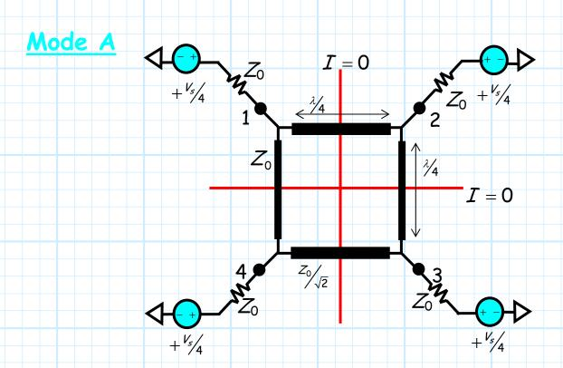
The even symmetry of this circuit is now restored, and so the voltages at each port are identical:
