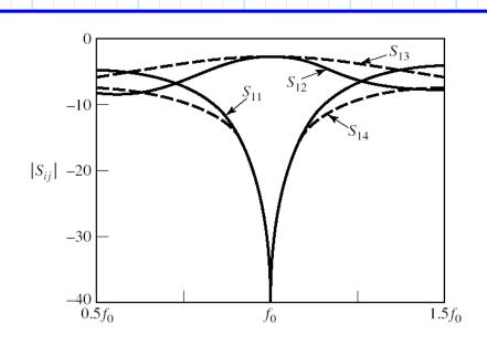
Figure 7.25 (p. 337)  ${\cal S}$  parameter magnitudes versus frequency for the branch-line coupler of Example 7.5
