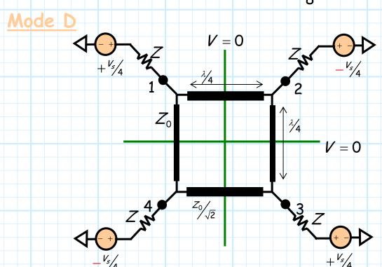
For mode D, odd symmetry exists about both planes of circuit symmetry.
