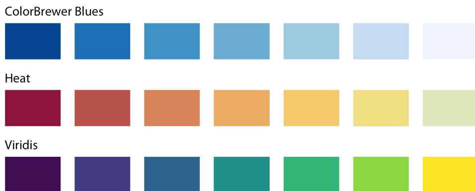
Figure 4-3. Example sequential color scales. The ColorBrewer Blues scale is a monochromatic scale that varies from dark to light blue. The Heat and Viridis scales are multihue scales that vary from dark red to light yellow and from dark blue via green to light yellow, respectively.
