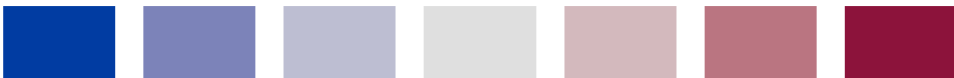
Figure 4-5. Example diverging color scales. Diverging scales can be thought of as two sequential scales stitched together at a common midpoint color. Common color choices for diverging scales include brown to greenish blue, pink to yellow-green, and blue to red.
