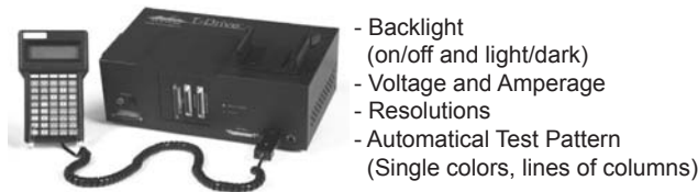
Figure 16. “T-Drive” for LCD module testing.
