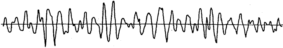
Fig. 12.8. Character of real wave shape (profile) to compare with ideal sine waves of Figs. 12.1 and 12.2. Note that the vertical scale is much exaggerated as before.
