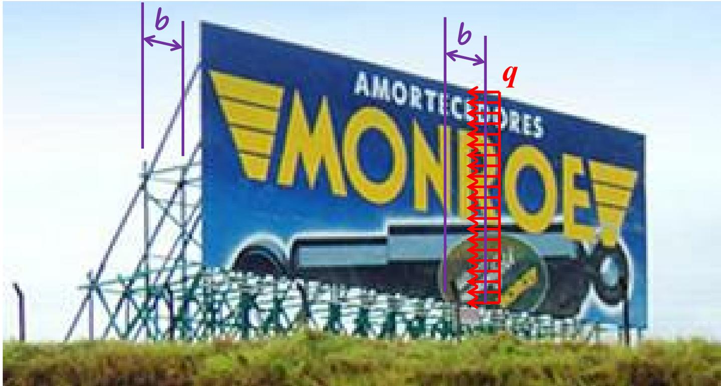
$$q = p \times b = 1,0 \frac{\text{kN}}{\text{m}^2} \times 2,6\text{m} = 2,6 \frac{\text{kN}}{\text{m}}$$
