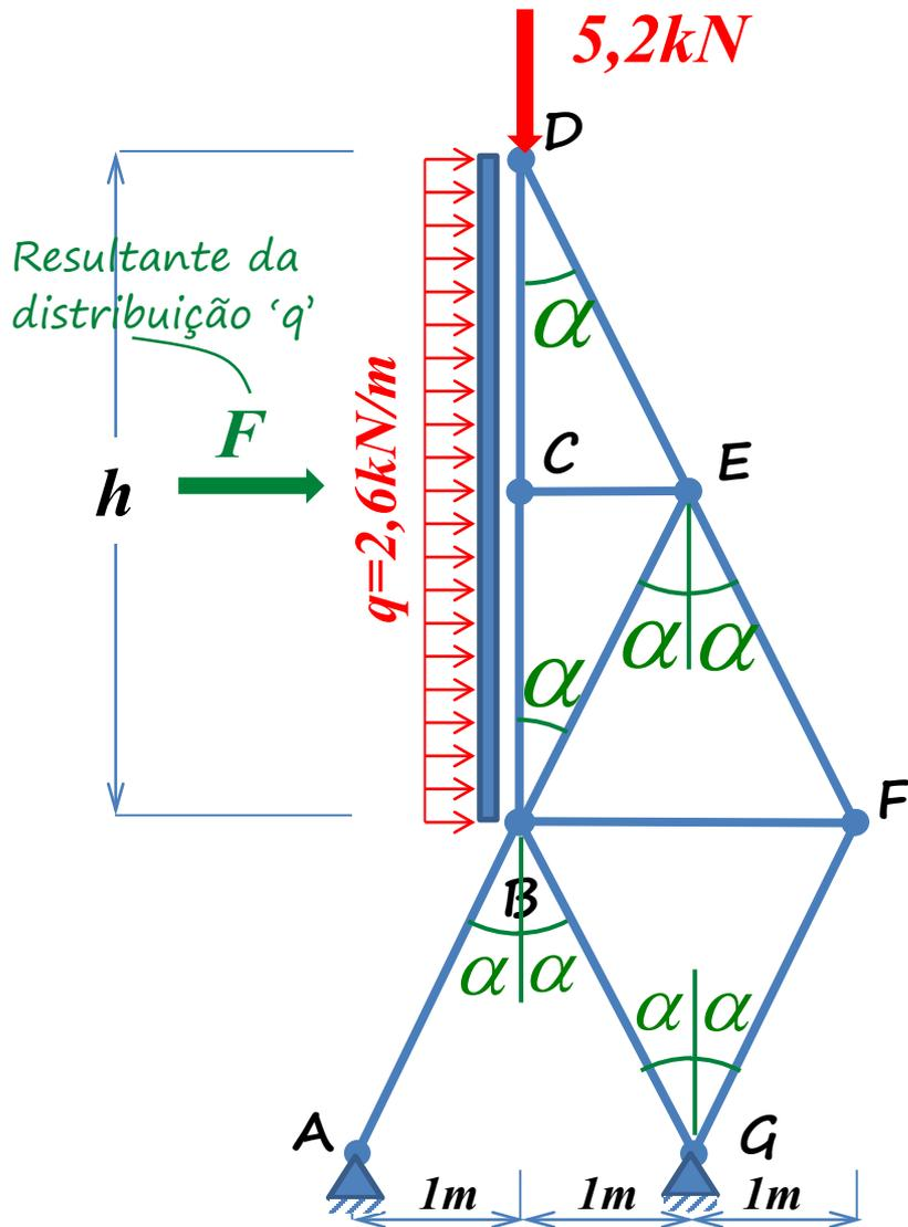
$$F = q \times h = 2,6 \frac{\text{kN}}{\text{m}} \times 4\text{m} = 10,4 \text{kN}$$
