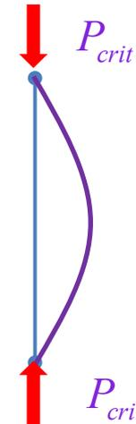
$$I \geq \frac{2 \times (\sqrt{5})^2 \times 26,162 \times 10^3}{\pi^2 \times 210 \times 10^9} = 1,26 \times 10^{-7} \text{ m}^4$$
