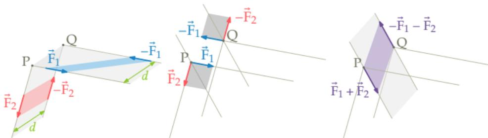
$$\vec{M} = (P - Q) \wedge (\vec{F}_1 + \vec{F}_2) = (P - Q) \wedge \vec{F}_1 + (P - Q) \wedge \vec{F}_2 = \vec{M}_1 + \vec{M}_2$$
