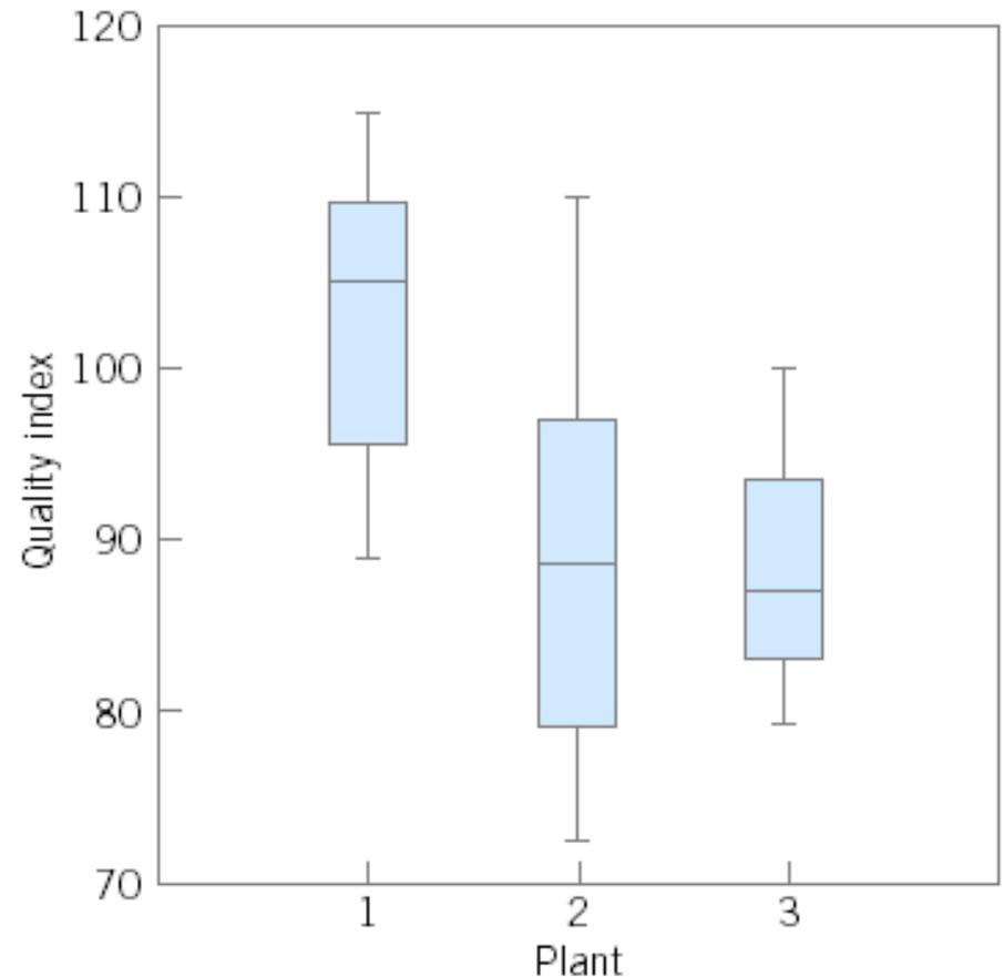
**Figure 2-8** Comparative box plots of a quality index for products produced at three plants.
