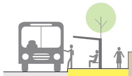
level Bus stops should be at the same level as the footpath and have proper gradient for surface runoff to avoid water logging especially during monsoons.
