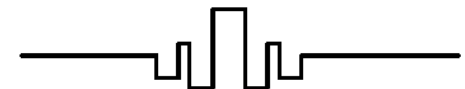
Up-and-down profile singlemode fibre (used in dispersion flattened fibre) also called multicladding fibre
