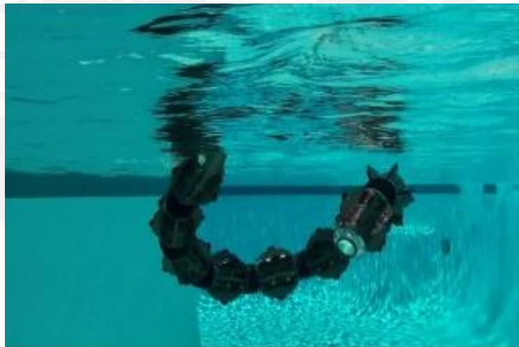
Figura 1.3.2.3. ACM-R5H. Fuente: http://www.hibot.co.jp/en/products/robots_1/acm-r5h_33
