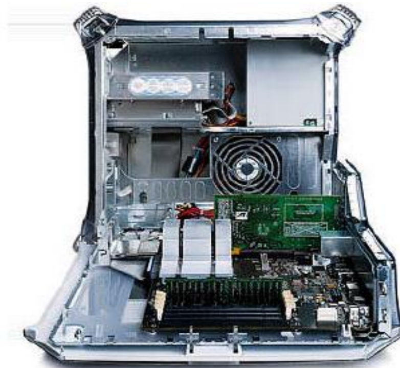
Figure 1. Swing-open door allows easy access to all components for upgrading and servicing
