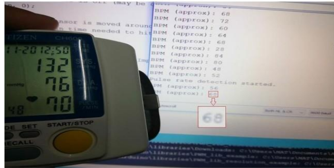
Figure 4. Pulse sensor output vs. Digital Blood pressure sensor
