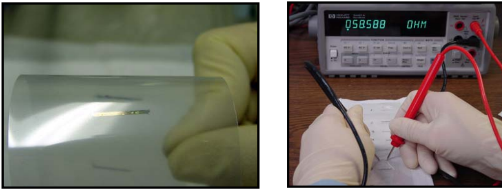
Figure 2.10: Inkjet printed gold lines on DuPont Melinex ® PET polyester film
