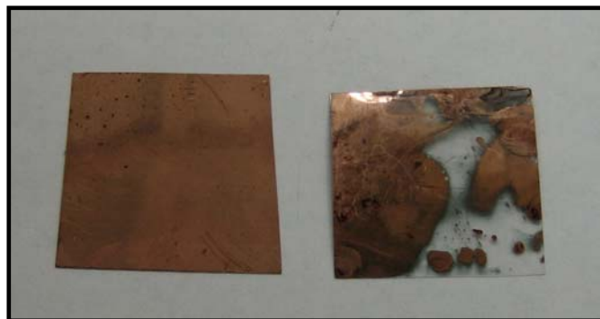
Figure 3.7: Effect of the corona treatment on electroless copper deposition (left: corona treated sample, right: without surface modification)
