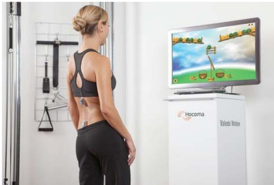
Figure 7 The Valedo low back pain therapy system by Hocoma AG combines wireless wearable motion sensors with interactive games to provide an engaging way to perform therapeutic exercises. Patients can set therapy goals, receive feedback on their performance and keep track of their progress. (Courtesy of Hocoma, Switzerland).
