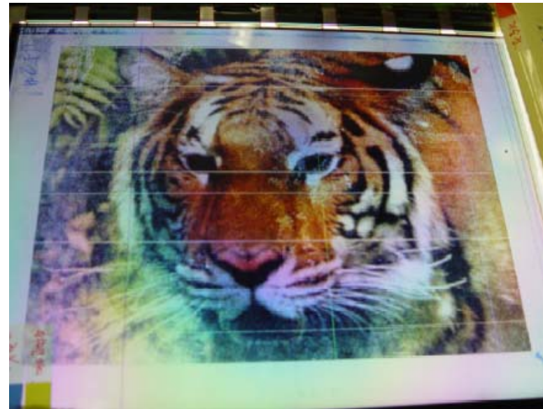
Prototype of 15" XGA OTFT-LCD
