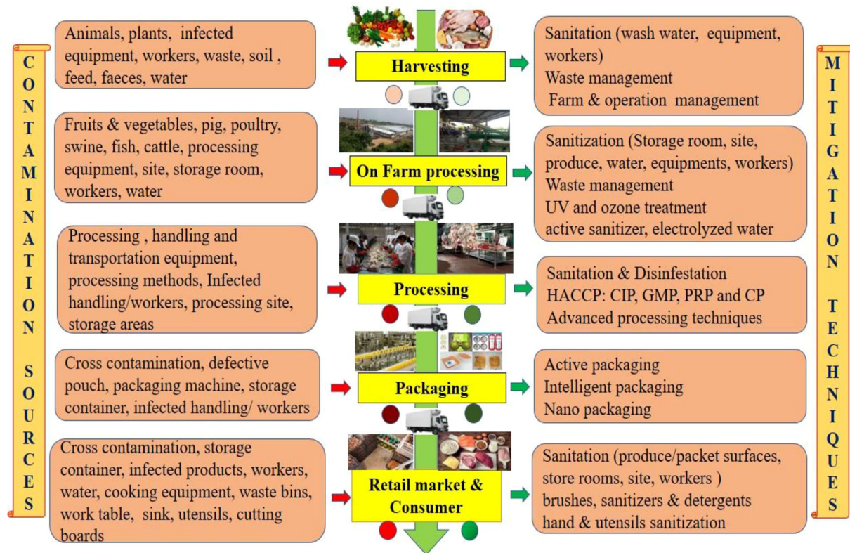
FIGURE 2 Various sources of contamination and mitigation techniques at different steps of the food chain. Source: Pérez-Rodríguez & Mercanoglu Taban (2019) and Al-Tayyar et al. (2020)
