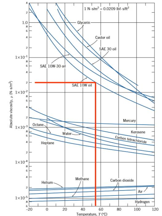
Fig. A.2 Dynamic (absolute) viscosity of common fluids as a function of temperature. (Data from References [1, 6, and 10].)
