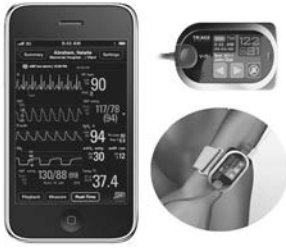
FIGURE 4.2: Airstrip Technologies' display of patient vital signs on a smart phone and the Sotera wrist transceiver, which directly displays the vital signs from the patient.
