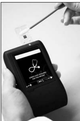
FIGURE 8.3: Prototype of a handheld genotyping and sequencing device.
