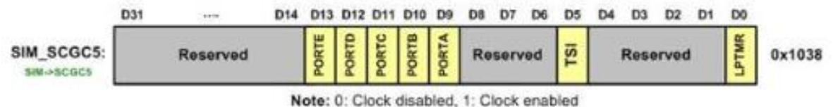
Figure 2-13: SIM\_SCGC5 (System Clock Gating Control Register 5) Register
