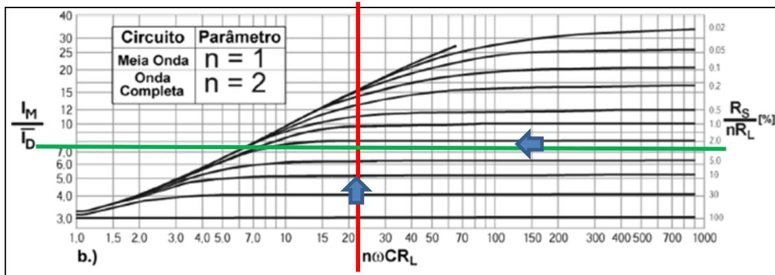
$$R_S/nR_L = 3 \% \text{ e } [n\omega CR_L] \cong 22 \longrightarrow I_M \cong 7,5 \times \overline{I_D} = 7,5 \times 0,7246 = 5,43 \text{ [A]}$$
