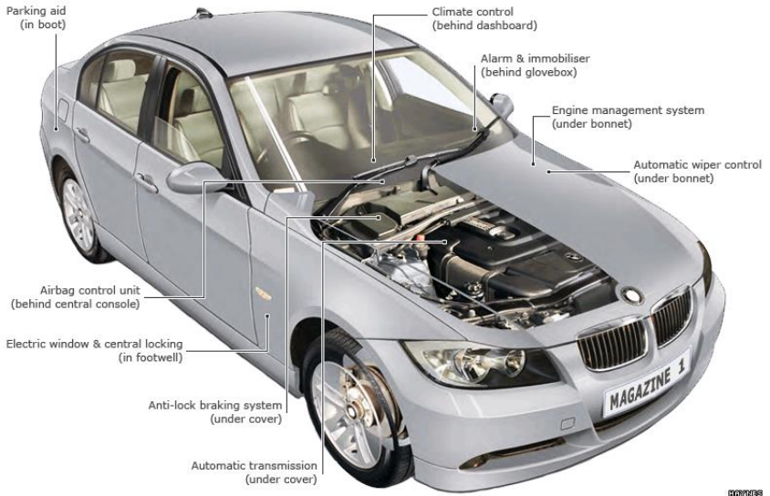
Fig. 1. Location of typical ECU's in a car (Magazine, 2010)
