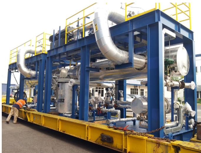
FIG. 7.2 Vacuum system of 100,000 L per day capacity AQUA SEP™, VOC SEP™ hybrid pervaporation and membrane distillation plant for nitrates, solvents and water purification.
