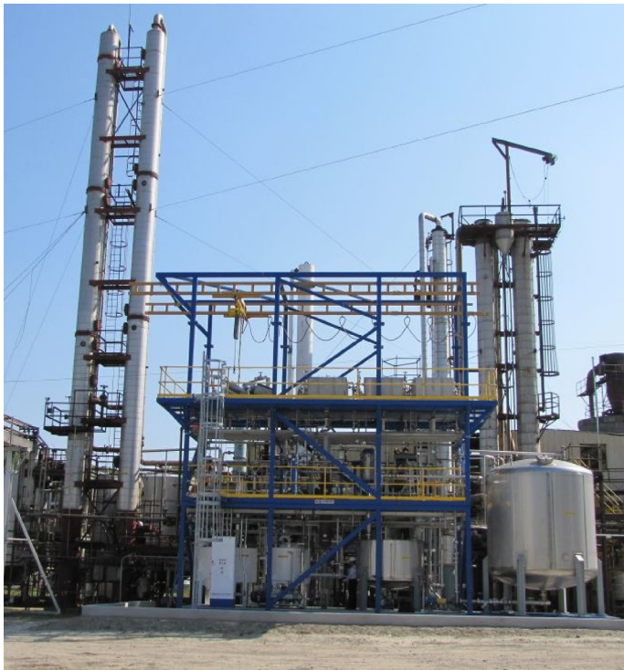
FIG. 7.9 40,000 L per day capacity AZEO SEP™ pervaporation plant for solvent dehydration.
