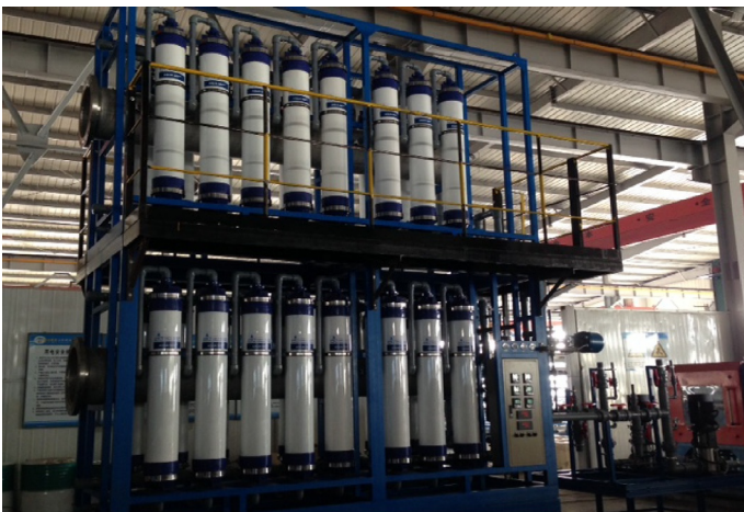
FIG. 7.11 VOC SEP™/AQUA SEP™ HYBRID hollow fiber plant to treat 100,000 L water/day.
