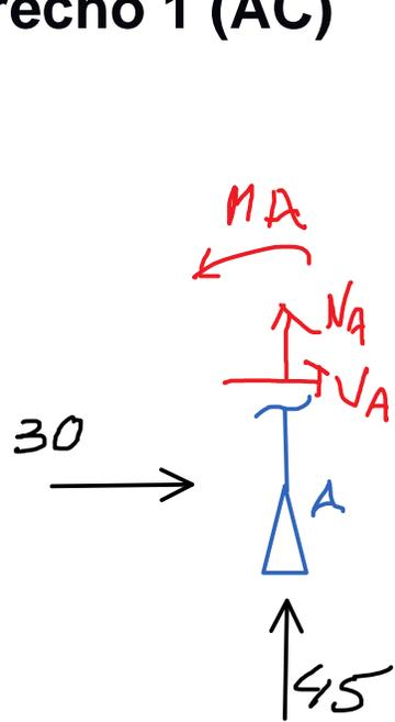
$$\begin{aligned}N_A &= -45 \\V_A &= -30 \\M_A &= 0\end{aligned}$$
