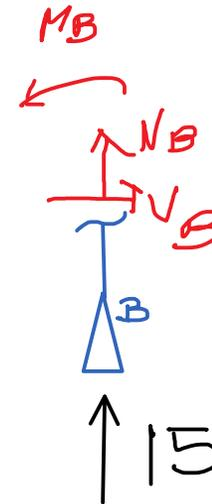
$$\begin{aligned}N_B &= -15 \\V_B &= 0 \\M_B &= 0\end{aligned}$$
