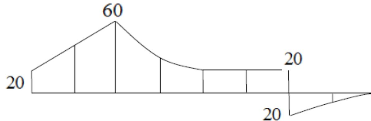
$$\frac{dN(x)}{dx} = -p_x(x) \quad \frac{dV(x)}{dx} = -p(x) \quad \frac{d^2M(x)}{dx^2} = -p(x) \quad \frac{dM(x)}{dx} = V(x)$$
