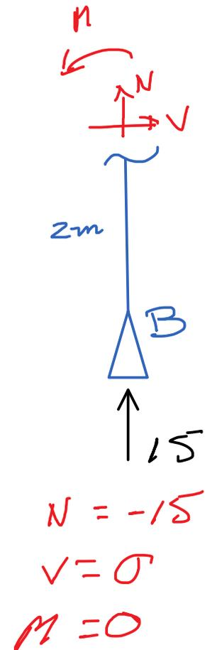
$$\begin{aligned}N &= -15 \\V &= 0 \\M &= 0\end{aligned}$$
