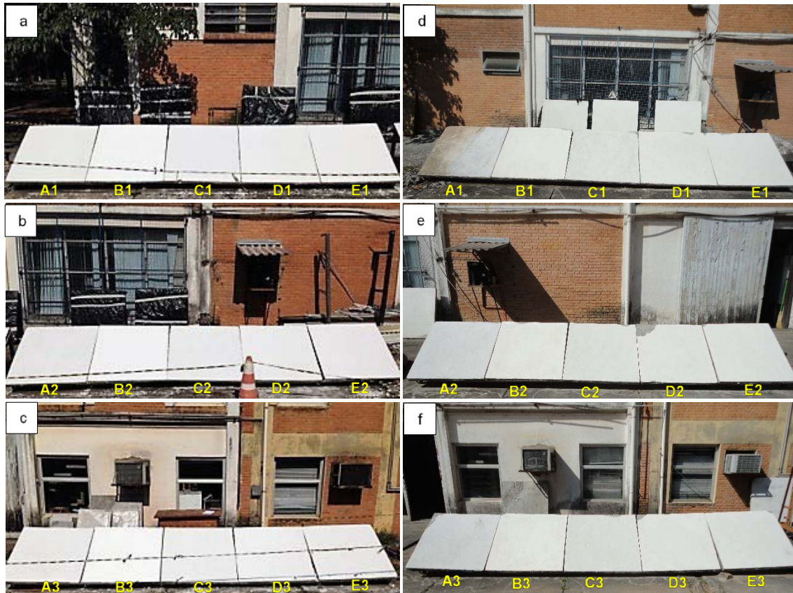
Fig.12: Color perception of specimens: (a,b, and c) 1 st month and (d,e, and f) 41 st month
