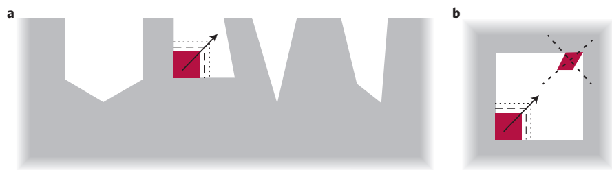
Figure 2 | Nucleation of crystals (red) in porous surfaces (pores, white; surface, grey). a , In a disordered, porous or pitted material, the large variety of pore sizes and shapes makes it highly probable that the nucleus of any polymorph will fit almost perfectly into at least one pore. b , In square pores, a cubic crystal is expected to nucleate faster than a triclinic polymorph (which has no right angles) because a cubic nucleus better fits into the right-angled corners of the square pores.
