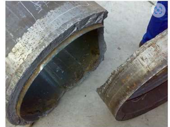
The hydrogen-induced cracking failure of an API 5L X60 line pipe.
