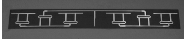
FIGURE 7.24 Photograph of an eight-way microstrip power divider for an array antenna feed network at 1.26 GHz. The circuit uses six quadrature hybrids in a Bailey configuration for unequal power division ratios (see Problem 7.33). Courtesy of ProSensing, Inc., Amherst, Mass.
