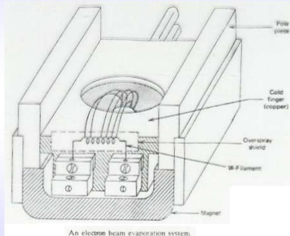
An electron beam evaporation system
