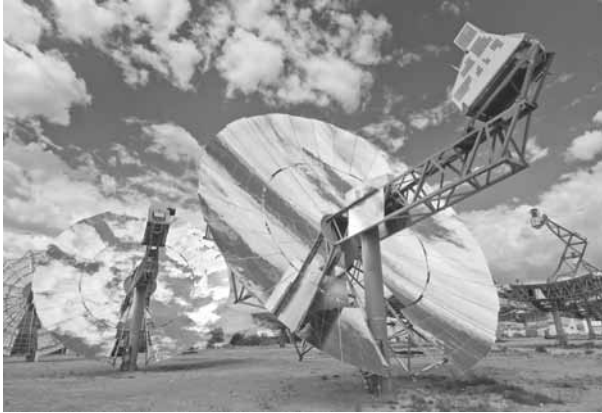
9.10 Stirling Energy Systems new 25 kW concentrator (SunCatcher) (Copyright: Sandia National Laboratories/Randy Montoya).
