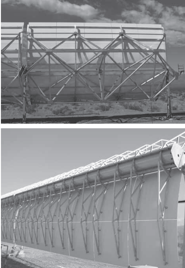
7.7 PTC designs using a space frame (top) and torque tube (bottom) to provide good torsional rigidity.
