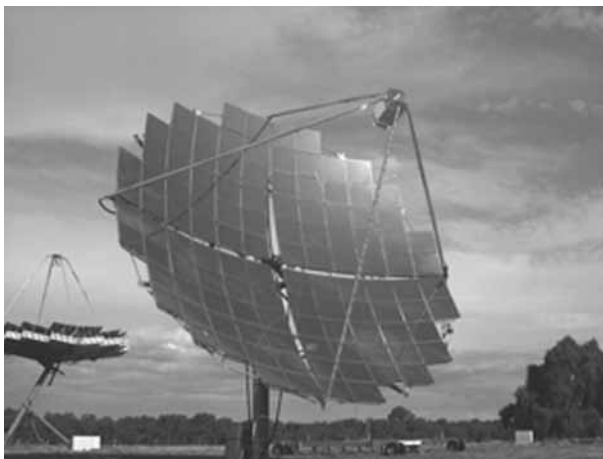
9.14 Solar Systems CS500 Dense Array CPV dish system.
