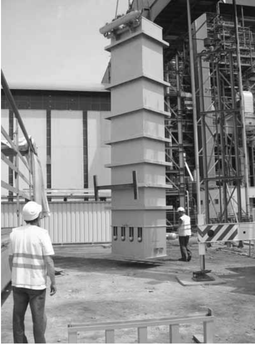
11.14 PCM storage unit using fins made of aluminium, 700 kWh th thermal capacity, operated with steam at 100 bar, integrated into a test loop connected to the power plant Litoral of Endesa in Carboneras, Spain.
