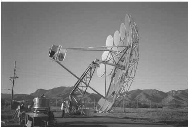
9.7 Cummins Power Generation CPG-460 concentrator.
