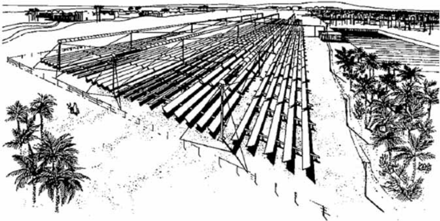
6.4 Sketch of a LFR solar plant in a desert environment (courtesy of Cesare Silvi, Italian Group for the History of Solar Energy (GSES) and the Italian Committee 'The History of Solar Energy' (CONASES)).
