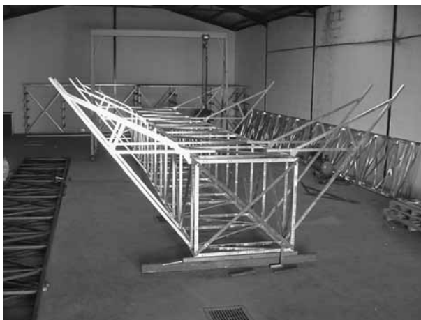
7.5 Steel structure of the Eurotrough-100 collector design.
