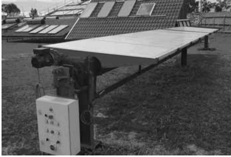
6.10 Prototype backbone and rib heliostat produced by Solahart in Perth in 1999 for the project (courtesy of Solahart Pty Ltd).
