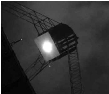
18.7 Image created on a diffuse cooled target by the Australian National University SG4 dish concentrator, with most of the dish reflective area covered in order to reduce the flux on the target (dark filters on the camera lens are used to make some of the focal region detail visible).
