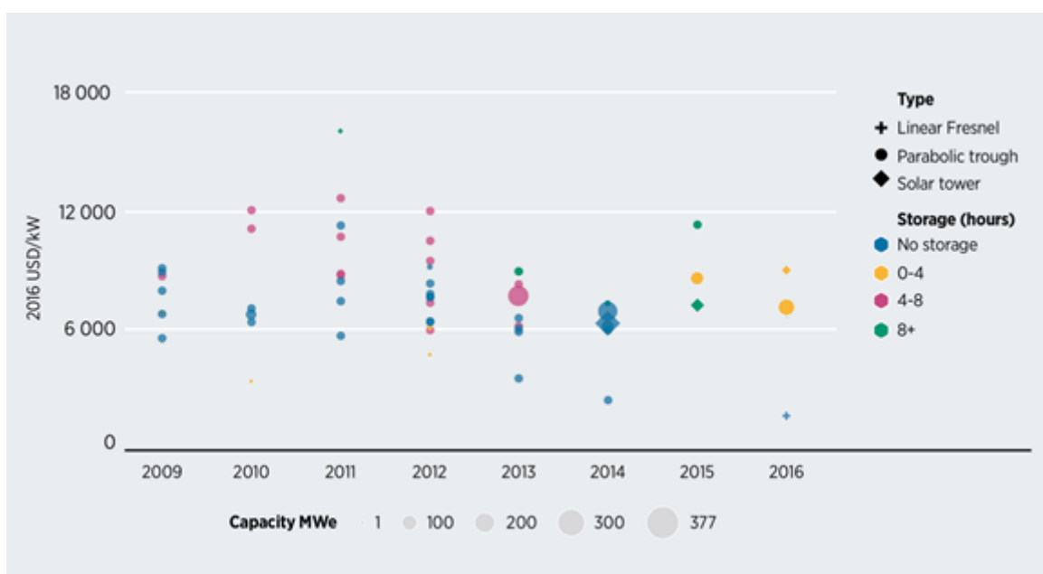
CSP installed costs by project size, collector type and amount of storage, 2009-2016. Source: International Renewable Energy Agency. [5]
