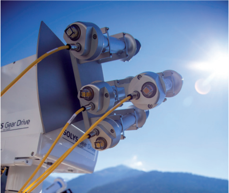
figure 33: automatic sun tracker with pyrheliometers
