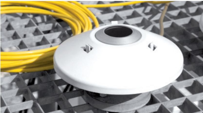
figure 37: pyrgeometer with meniscus dome
