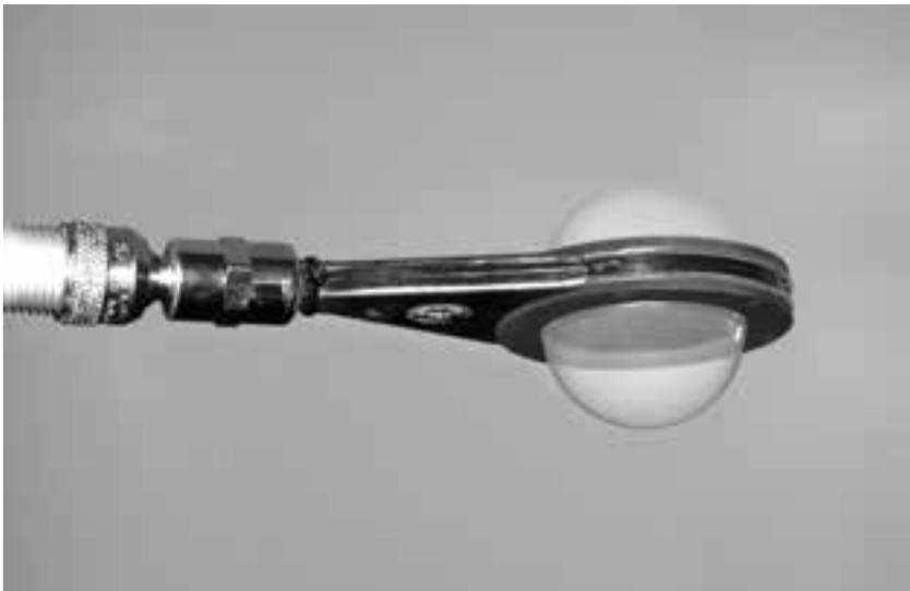
figure 20: REBS Q7.1 net radiometer with polyethylene domes
