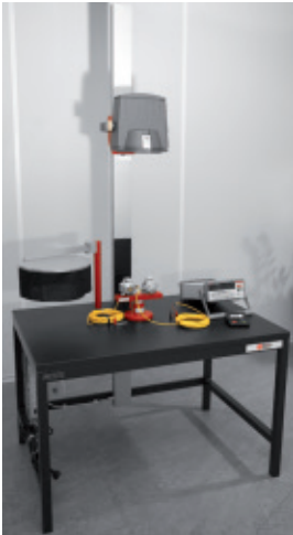
figure 26: calibration facility for pyranometers
