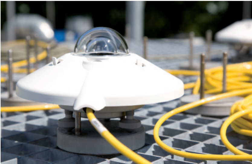
figure 21: pyranometer with sun screen
