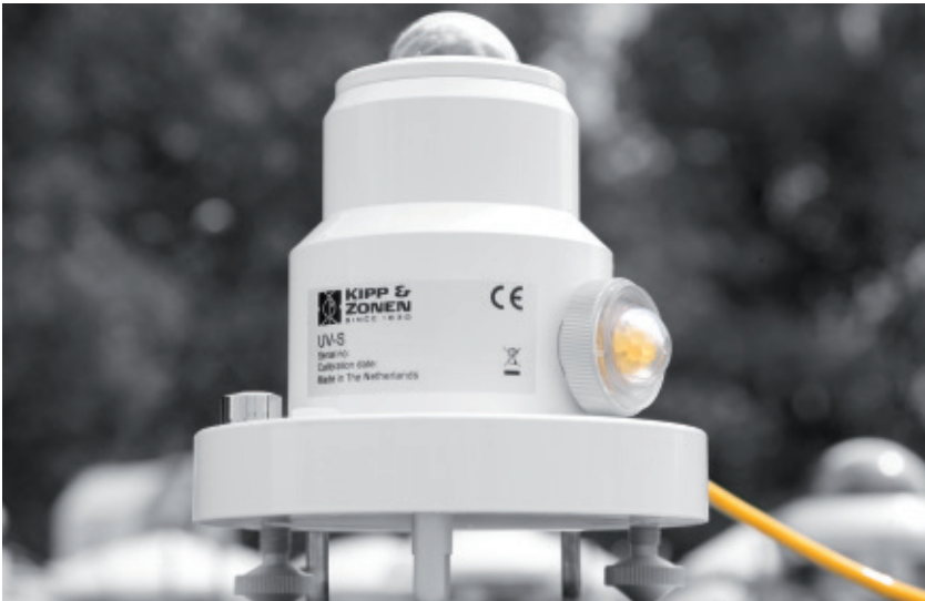
figure 53: UV sensor with specific spectral response (UVA, UVB or UVE)
