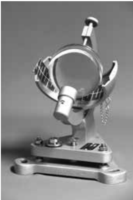
figure 56: Campbell-Stokes sunshine recorder (image by Thies Clima, Göttingen, Germany)
