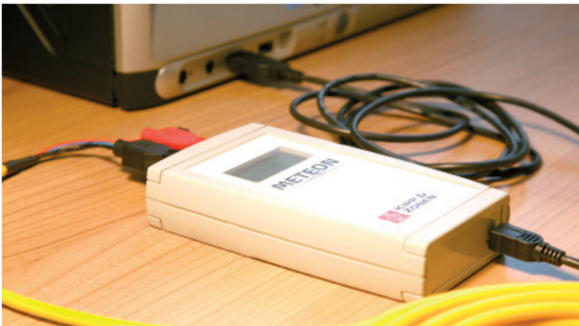
figure 74: hand-held irradiance meter and data logger
