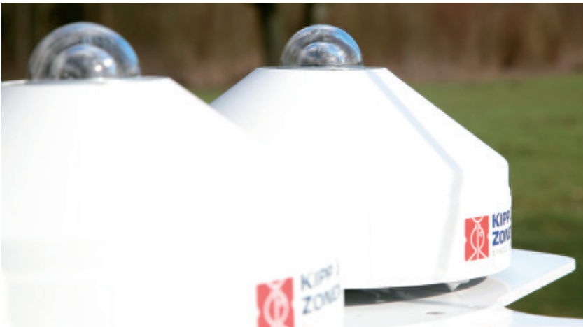
figure 66: ventilation units fitted to pyranometers
