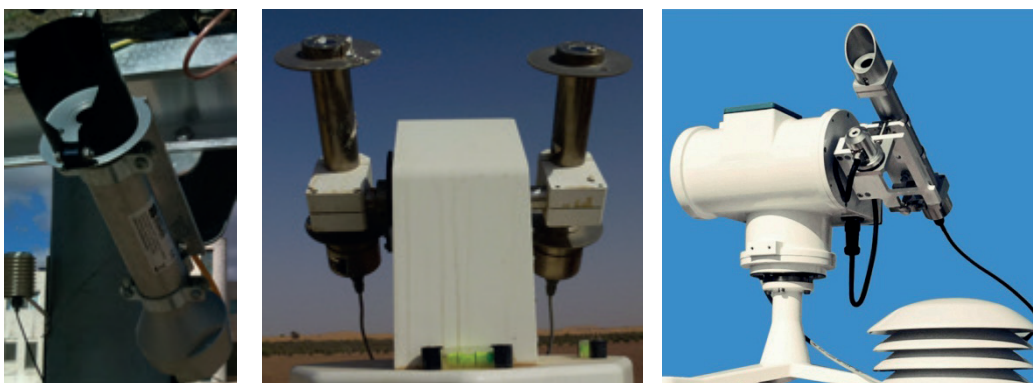
Figure 3: Thermopile pyrheliometer instrument (Left: Kipp & Zonen CHP1; center: Eppley solar tracker with two arms for pyrheliometers; right: EKO Tracker with Hukseflux DR02-T1). © Suntrace (2015)
