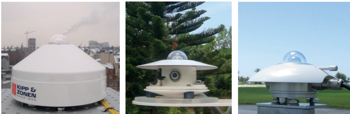
Figure 4: Examples of thermopile pyranometers (Left: Kipp & Zonen CHP21, center: Eppley PSP, right: Hukseflux SR20-T1. © Suntrace (2015))
