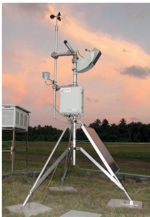
Figure 12: CSP-Tier 2 station with Rotating Shadowband Pyranometer mounted on a tripod, which is fixed on concrete slabs. © Suntrace (2015)
