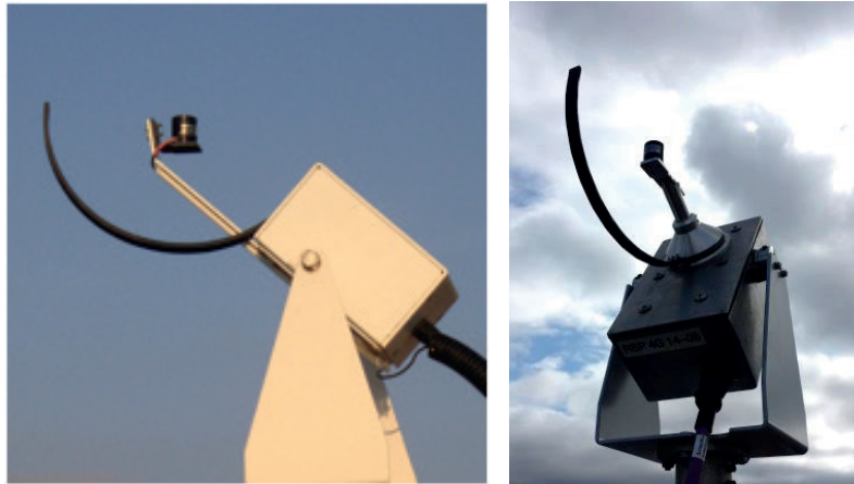
Figure 7: RSI instruments (left RSR2 of Irradiance Inc.; right RSP4G of Reichert GmbH). © Suntrace (2015)
