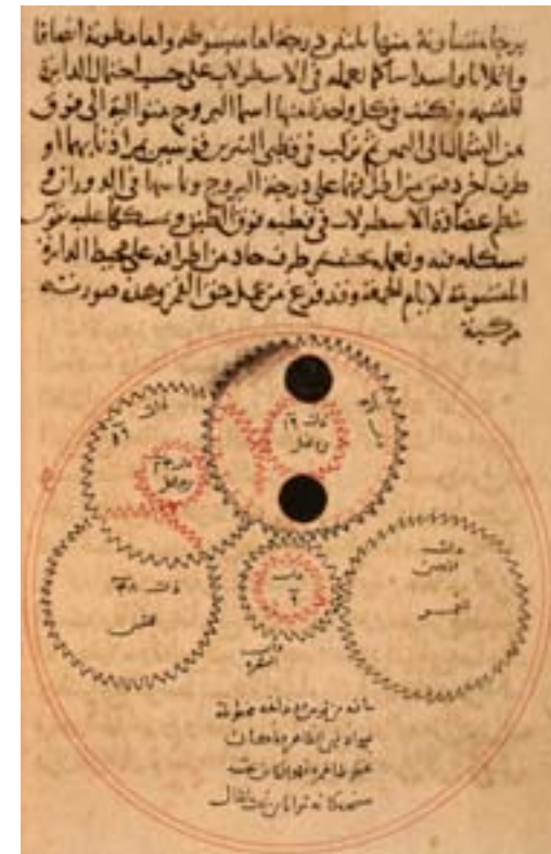
A page from one of only three known copies of a treatise by al-Biruni on astrolabes, a tool used to predict the positions of the sun, moon and planets. The illustration shows the internal gearing of this mechanical calendar and may be the first surviving work to illustrate such miniature technology.
